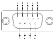
**DB9 pin definition for RTU-type UP-Hi series:**
