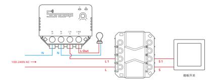
The wiring instruction of connecting the S-MATE with three MINIR3:
