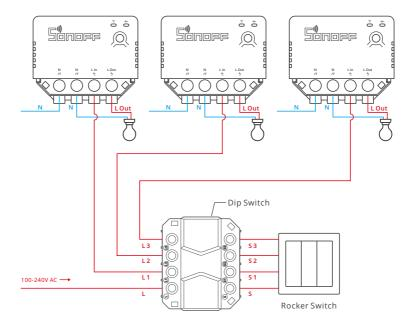
() The dip switch is factory set to the right. Please toggle the dip switch to the left if connection a pulse switch to the device.
