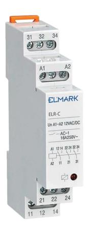
Intermediate Relays are used for switching larger load output, strengthen or multiplying contacts of the existing device or send signals to the relevant control elements concurrently. Relays from ELR-7 series are easy for operation and has different input voltages- from 12V DC, 24V AC/DC and 240V AC
