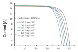
Voltage [V] Module characteristics at variable module temperatures and constant module irradiance of 1.000 W/m<sup>2</sup>
