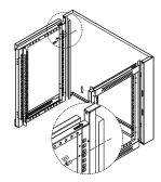
4 Use 4 of the included M6 screws (use 6 for larger units) to attach each of the 2 side frames (3) to the back frame (6).
