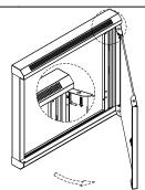
2 Use the included key to pull open the door (1) and remove it from the front frame (2) by pushing down on the latch.
