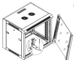
**R** Reverse Step 2 by inserting the lower door latch into the frame and then pushing down on the upper door latch to install the front door (1). Note: Once the unit is assembled, check that all corners are square to ensure that the door opens and closes properly.
